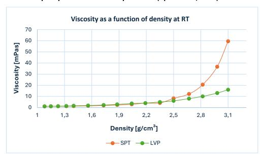
The high viscosity of sodium polytungstate solutions often leads to prolonged separation times for solids in the fine particle range and at high densities (> 2.8 g/cm³). Using laboratory centrifuges, the separation process can already be significantly accelerated. Our solution, however, provides a compelling alternative:
